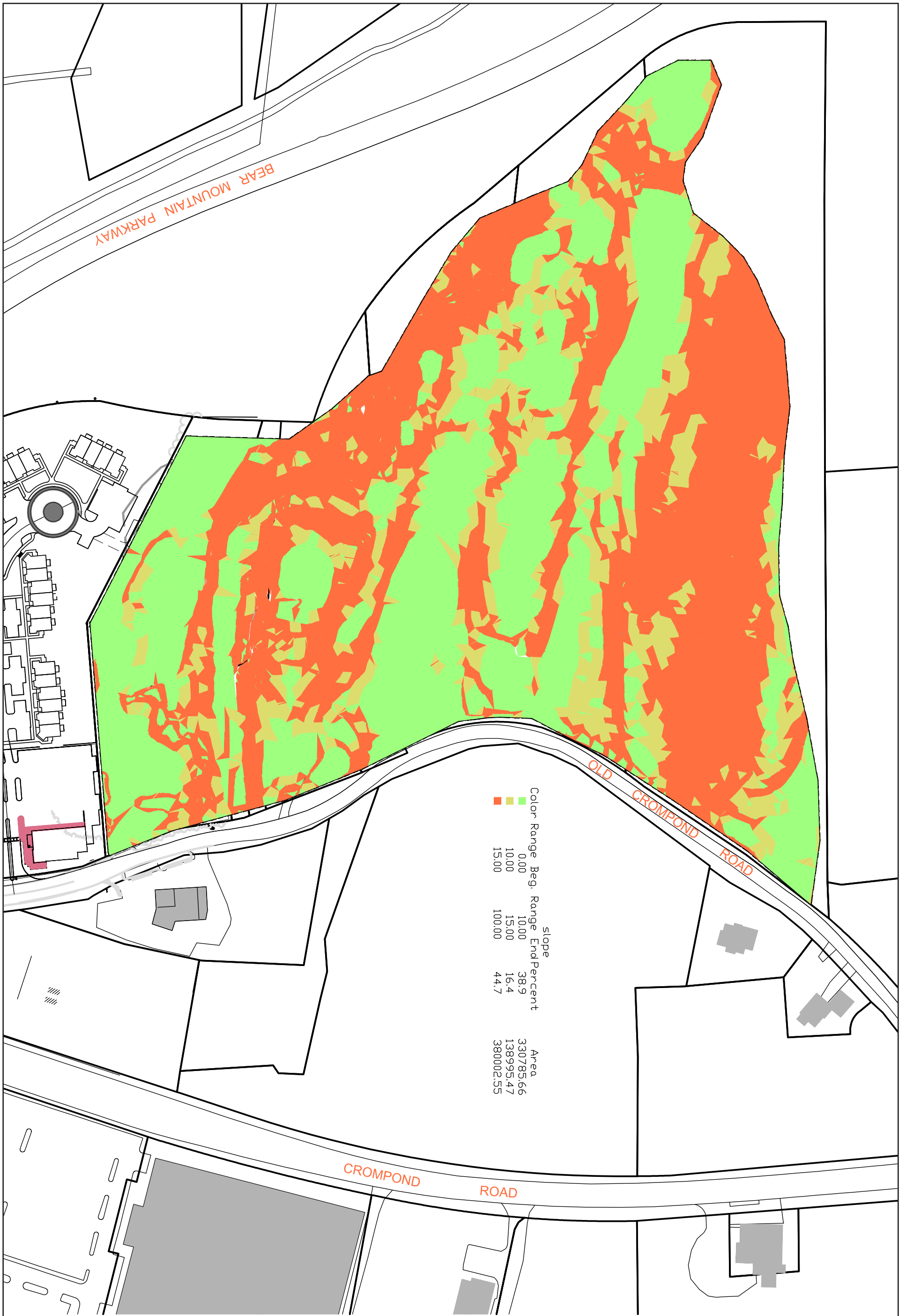
Figure 4-2: Slope Disturbance Map Bear Mountain Triangle Rezoning Town of Yorktown, New York Source: Ciarcia Engineering, P.C. Approx. Scale: 1" = 175'
